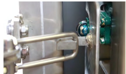
Safety switch prevents operation while door is open
